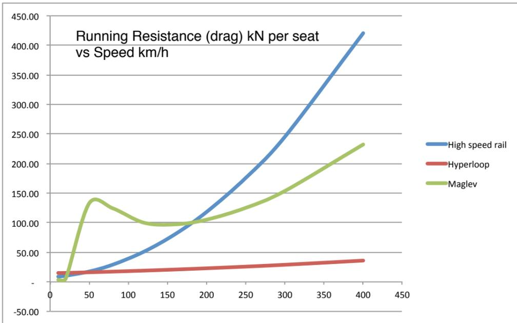
The chart shows the running resistance for the maglev and train, divided by the number of passengers seats so they can be compared. The maglev shows very high drag at lower speeds, reducing at high speeds compared to the HSR. The better high-speed drag might be due to the very clean aerodynamics of the Transrapid.
