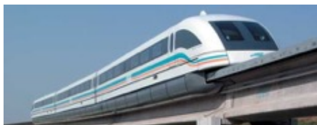
The Shanghai Transrapid train, the only high-speed maglev in service, with a 30km track.
