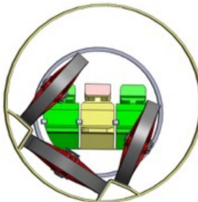
The banking angle of the rails is a manufacturing problem. It will take about 3 seconds to adopt the banking angle in a fast curve, that is about 1km of distance. The rails need to gently alter their angle for each 25m section of tube, which is a difficult machining operation with the required accuracy.
