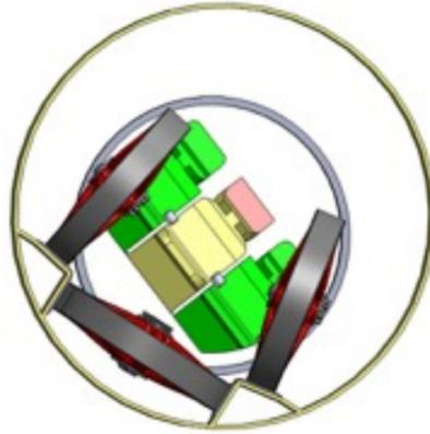
**At slow speed** in the same curve, due to a station, delays or maintenance, the passengers need little or no bank angle. But the rails are still angled at 30 degrees. So the seats need to angle down by up to 30 degrees.
