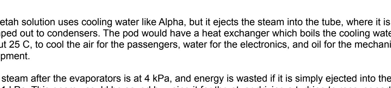
Cheetah solution uses cooling water like Alpha, but it ejects the steam into the tube, where it is pumped out to condensers. The pod would have a heat exchanger which boils the cooling water at about 25 C, to cool the air for the passengers, water for the electronics, and oil for the mechanical equipment.
