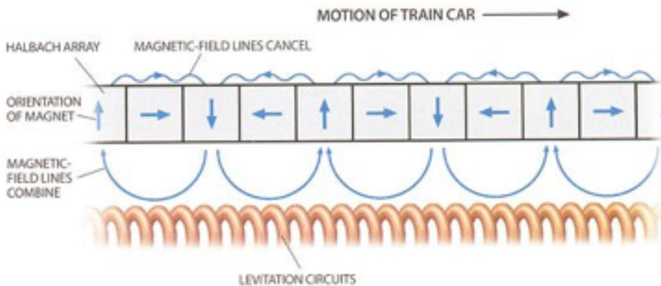
In the Pod Competition tube, the coils would be replaced by a simple aluminium plate
