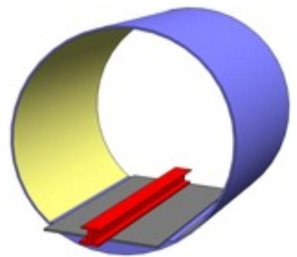
The low lift/drag ratio is inherent in the unsuitability of a plain conducting plate compared to copper coils. This type of maglev is impractical for a full-size Hyperloop system.
